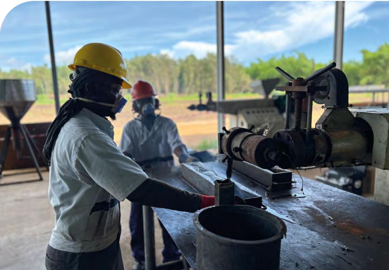
RecoPlast - Manufacturing of paving stones from plastic collected on beaches - May 2024 - Democratic Republic of the Congo
